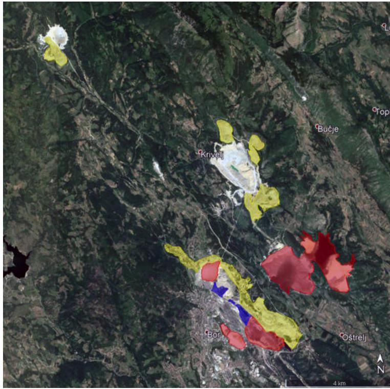
Figure 2. Bor copper mine (yellow – waste rocks and oxide ore tailings, red – flotation tailings, blue – metallurgical slag)
