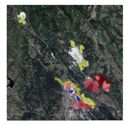
Figure 2. Bor copper mine (yellow – waste rocks and oxide ore tailings, red – flotation tailings, blue – metallurgical slag)
